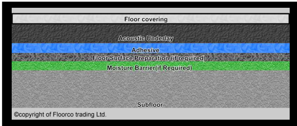
Floating SPC flooring
